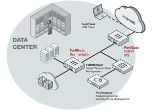
FortiGate 2200E deployment in data center (IPS/NGFW, Intent-based Segmentation)
